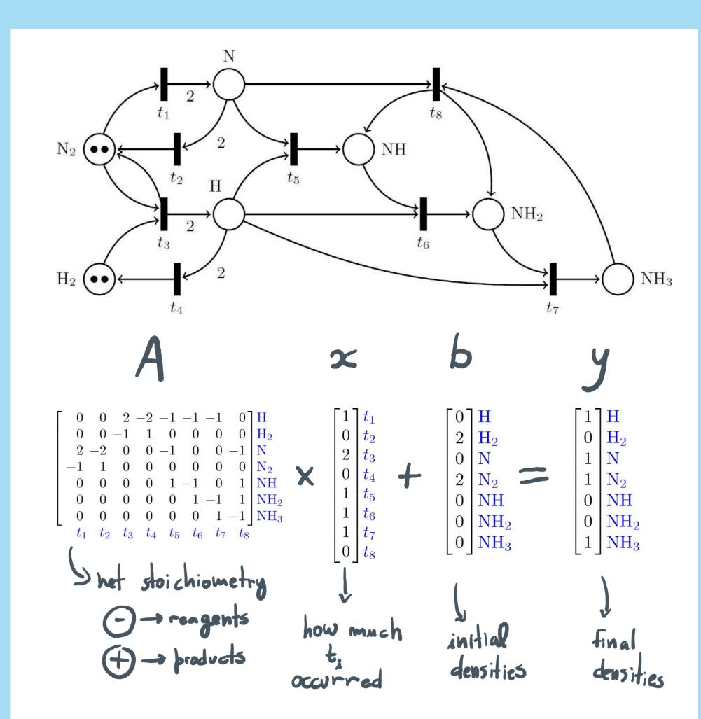
With the linear approximation Ax+b=y we consider the global transformation of the initial state densities b to the steady-state densities y. This final density y is compared with reference data from LoKI-B software[4], an electron Boltzmann equation solver for LTPs. Our goal is then to find the weights x that minimize this difference. Since these reaction weights represent pathway importance, we effectively reduce our original kinetic scheme by removing low-weight reactions.
