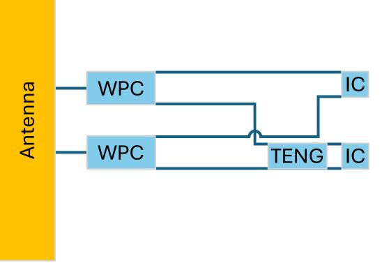
TENGs can introduce an impedance mismatch in the circuit to signal its on/off state. The twin-tag single antenna model was used with Wilkinson Power Combiners to equally divide the power between the two RFID ICs.
