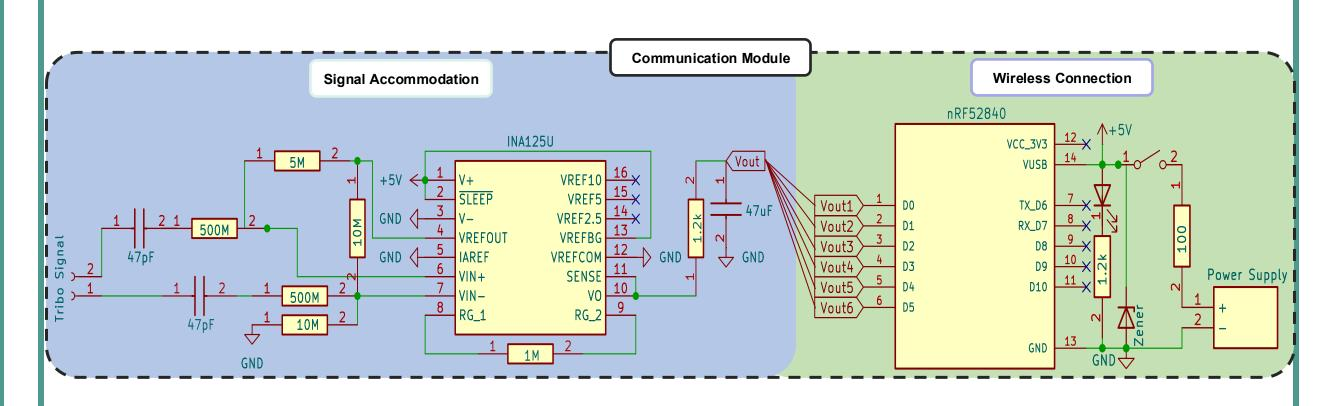
Circuit diagram of the communication module, showing the signal conditioning stage (blue) with impedance matching and noise reduction, and the wireless module (green) with Bluetooth Low Energy capabilities.
