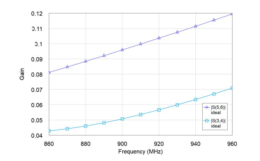
Simulation was performed using ports 3 and 4 (light blue), with impedance mismatch caused by the TENG sensor, and ports 5 and 6 (dark blue), for the unmodified branch.
